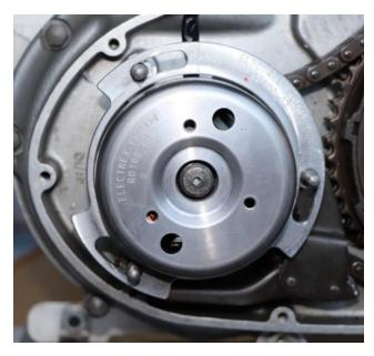
Then using the spacer and collect provided the rotor should not foul/hit the stator. The dished part of the rotor, where the fitting nut locates, should be level with the end of the crankshaft.
