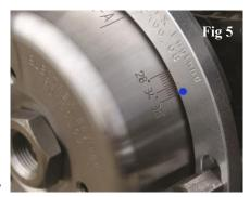
Tighten the rotor retaining nut to about 40Ft/lbs torque. Final adjustment can be made by moving the stator on the slotted holes - tighten the x3 nuts when set.
