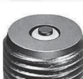
In a sense, this is the ultimate plug configuration. Nearly all insulator cracking and electrode melting can be prevented with this type. Nevertheless, service life and low-speed performance may suffer slightly.
